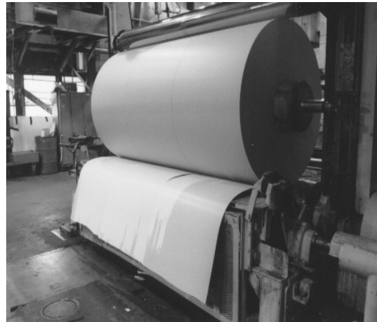
After drying the multi-layer fiber mat, it is coated and then rolled and slit to its final size.
