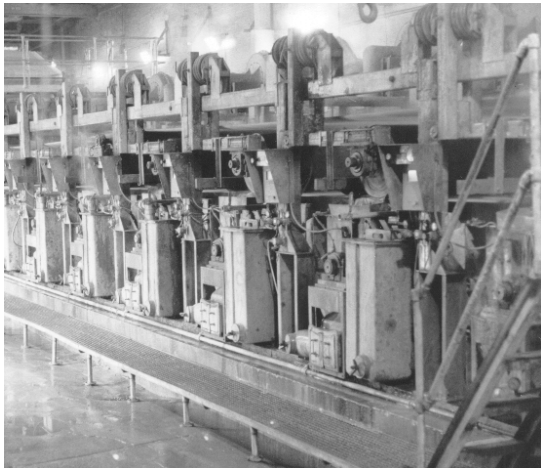
The paper machine receives the thin slurry, forms a mat by draining water, and transfers the mat to a felt.
